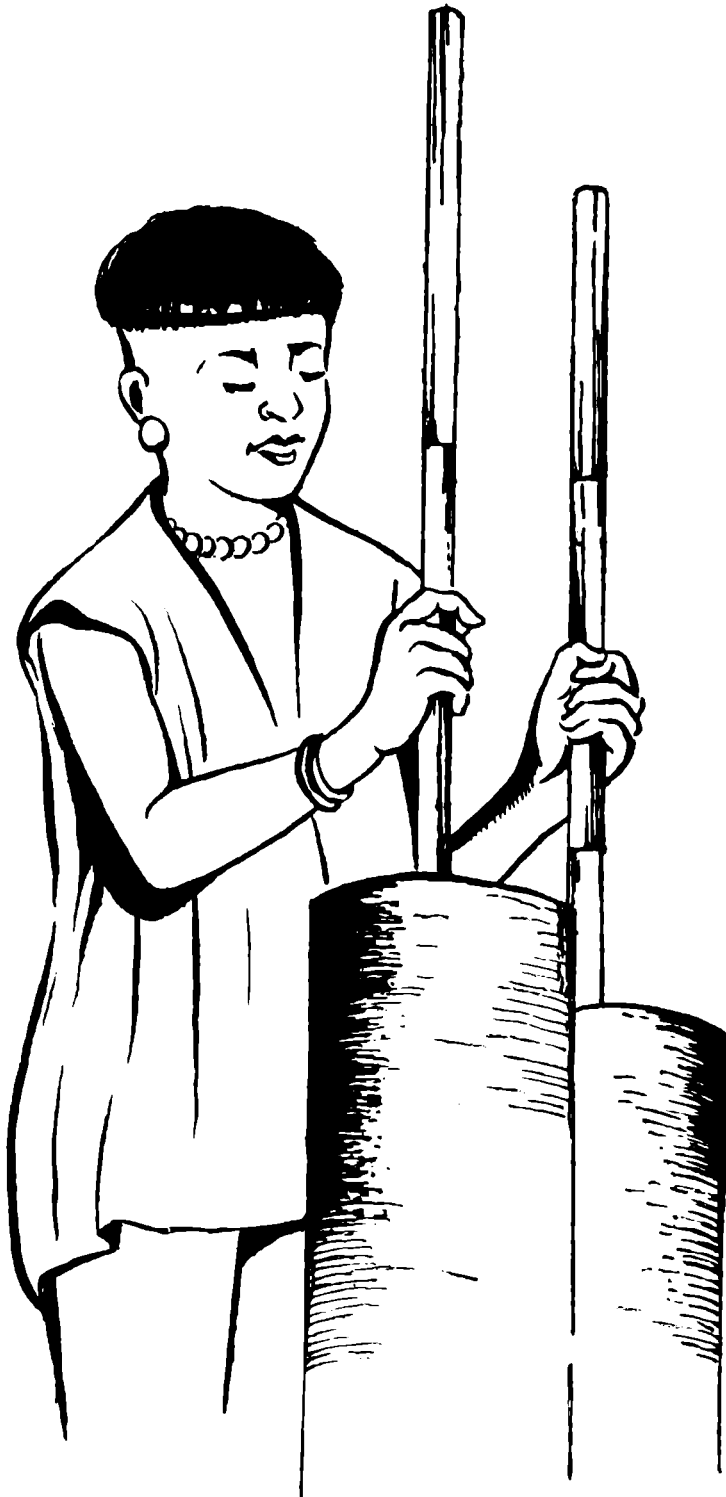
Double cylinder bellows in action
